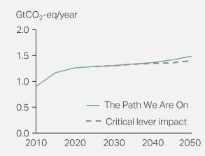
Strengthened energy efficiency has the most standalone emissions reduction impact in 2050 (~220Mt  $CO_2$ -eq/year). This is achieved by a lower total energy demand in the fleet due to more efficient vessels from regulatory tightening rather than transitioning to alternative fuels
